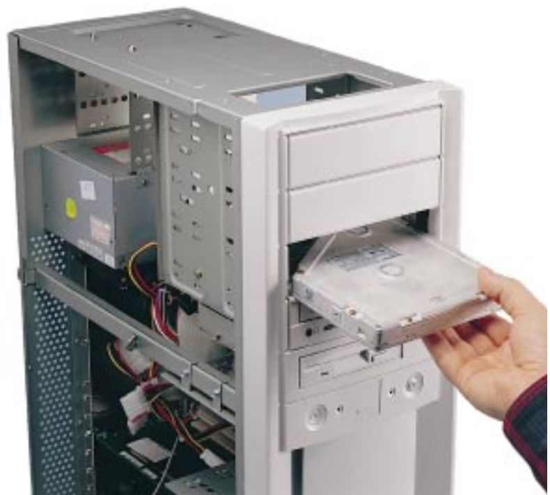
Fig 1 It's easier to slide the new hard drive into one of your PC's forward-facing bays. However, installing it inside the case, perhaps under the floppy drive, leaves more room for extra devices
